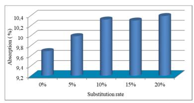
Fig. 9. Variation of absorption by immersion versus the substitution rate
