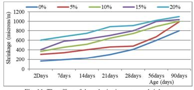
Fig. 11. The effect of the substitution rate on shrinkage
