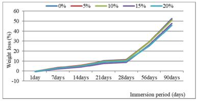
Fig. 13. Variation of weight loss versus the immersion period in H<sub>2</sub>SO<sub>4</sub>
