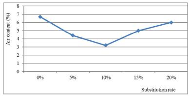
Fig. 4. Change in air content as a function of the substitution rate
