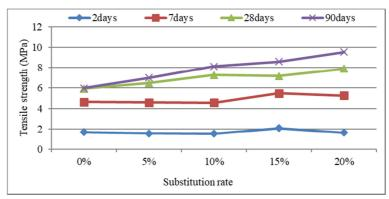
Fig. 8. The effect of age on the development of tensile strength
